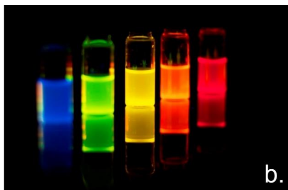
Figure 1: Nanocrystals as light source. a. Luminous efficiency of various light emitting technology over the years. AI generated graph. b. Image of a set of colloidal quantum dots with various size as synthesized at ESPCI.
